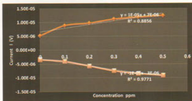
Cyclic voltammogram of methylamine in different concentrations and the bottom is the peak current response at different concentrations. Upper line shows the oxidation response and the bottom due to the reduction.
