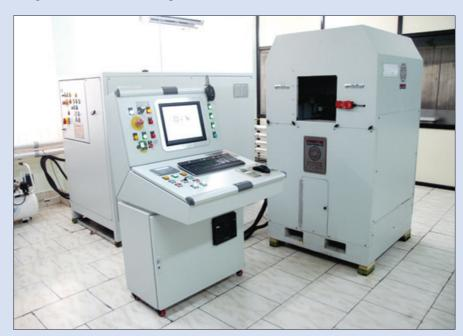
High Pressure Processing Equipment installed at CIFT and procured from M/s Stansted Fluid Power Limited, United Kingdom
