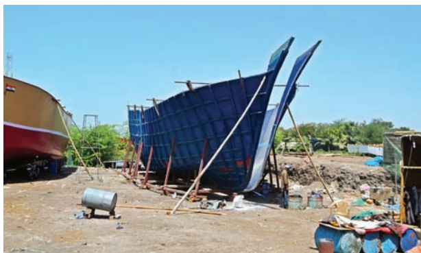
Mould used for FRP Boat construction and inner wooden ribs of FRP boat
