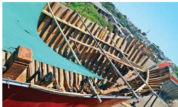
Mould used for FRP Boat construction and inner wooden ribs of FRP boat
