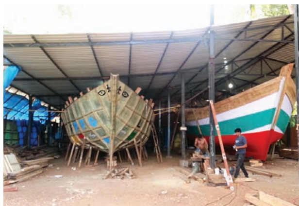
Fig. 1. FRP boat building yard at Devgad
