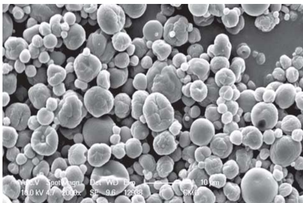
Fig.1. SEM image of microencapsulated fish oil prepared without oregano essential oil (CHGM)
