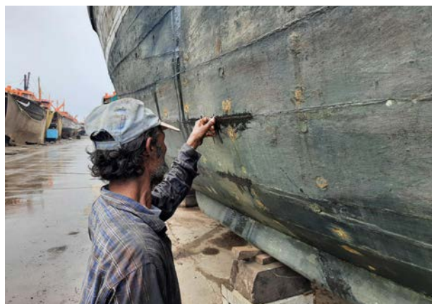
Fig. 2 Mixing and application of Damar Batu
