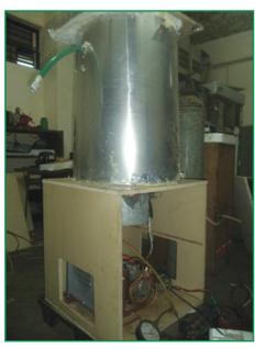
Water chilling unit using solar energy
