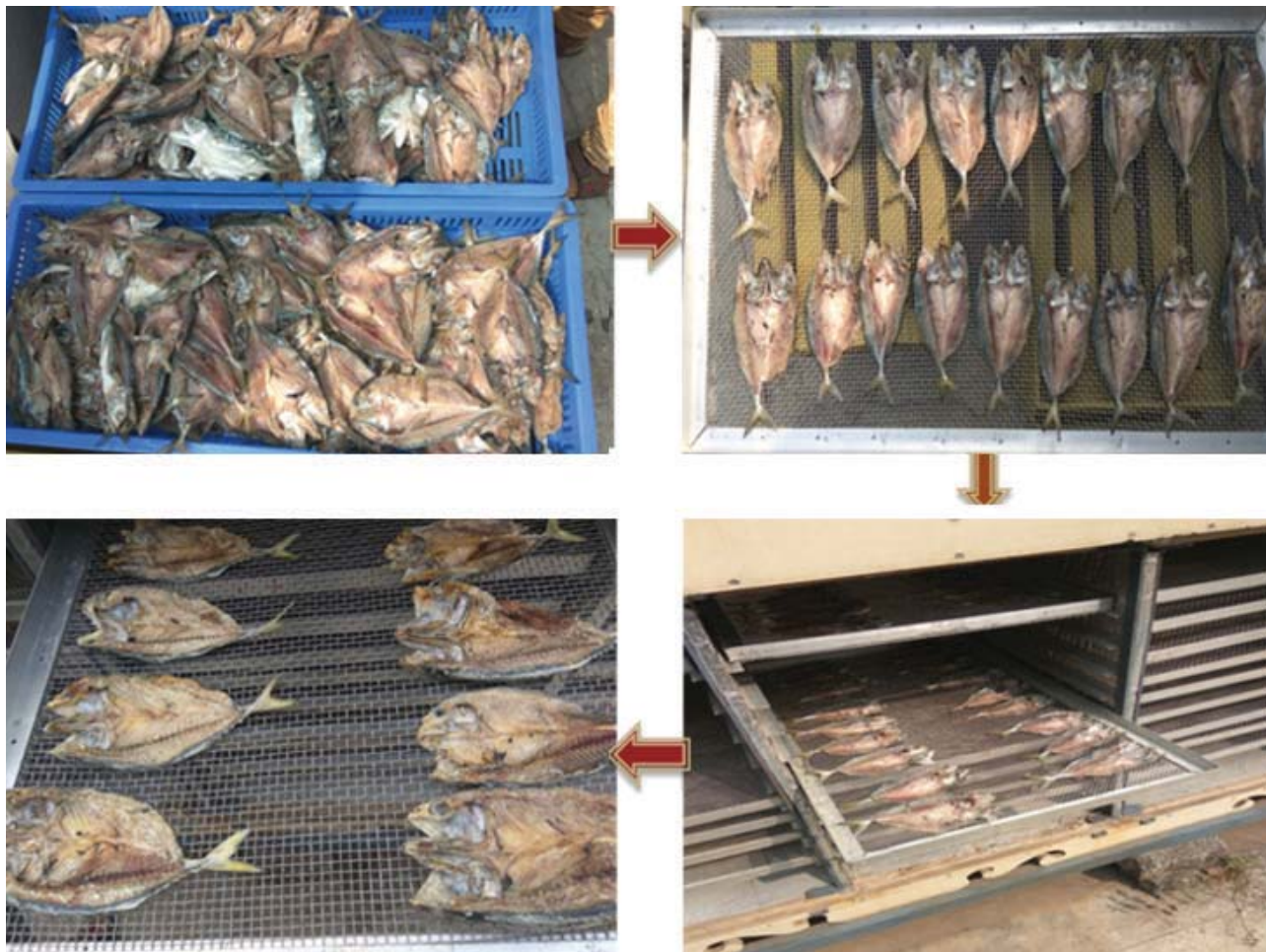
Drying process flow of mackerel fish in ICAR-CIFT solar dryer
