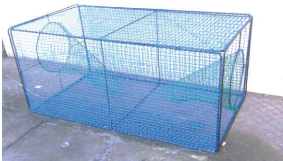
Modified collapsible trap for capture of Pearlsport
