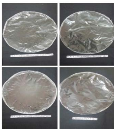
Virgin PLA and PLA/nanochitosan cast films in different concentrations
