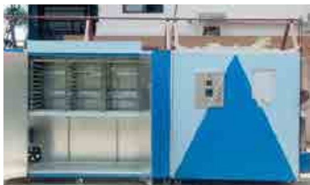
Redesigned ICAR-CIFT solar-LPG hybrid dryer
