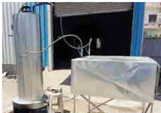
Mini boiler with steaming chamber (Hybrid: Biomass + LPG)
