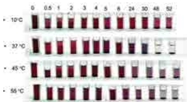
Gold nano particles showing colour change upon temperature abuse from frozen storage condition
