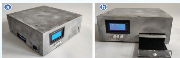
3D printed fish freshness sensor (a) Isometric view (b) Front view with open tray
