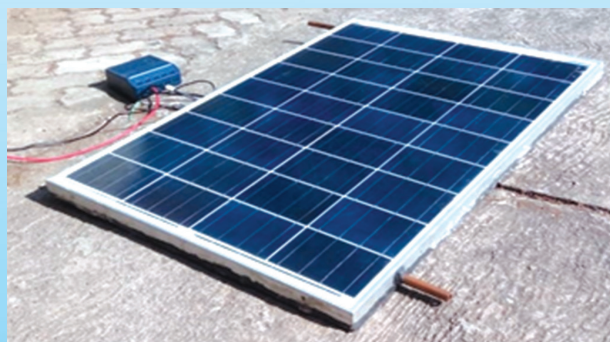
Photograph of developed hybrid photovoltaic panel (PVT) with charge controller.
