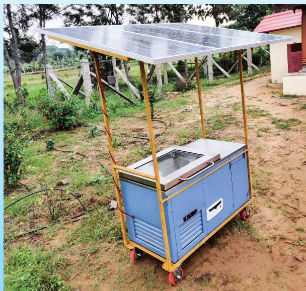
Solar powered refrigerated mobile fish vending kiosk under field evaluation
