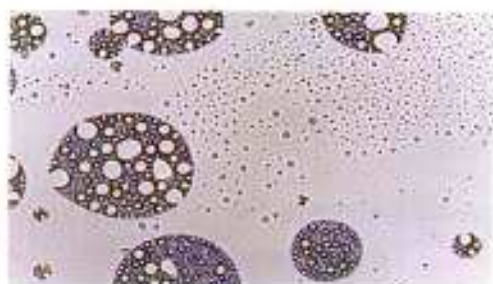
Emulsion microstructure of water in oil in water (W/O/W) emulsion
